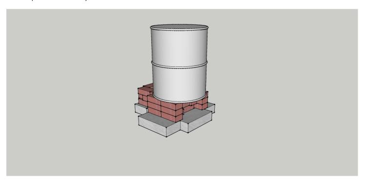
Cut away view of barrel placement. Barrel is 22" diameter, 28" tall
