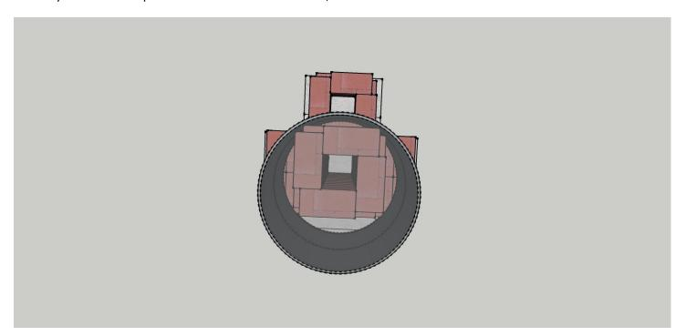
Top of Chimney is 1  $\frac{1}{2}$ " below top of barrel
