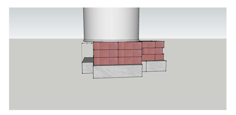
Edge of barrel is 7  $\frac{1}{2}$ " from edge of chimney.
